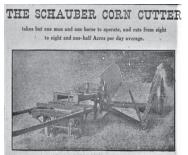
The Corn Cutter was pulled by a horse from one end of the field to the other. A knife made of cutlery steel was drawn just above the ground cutting through the corn
